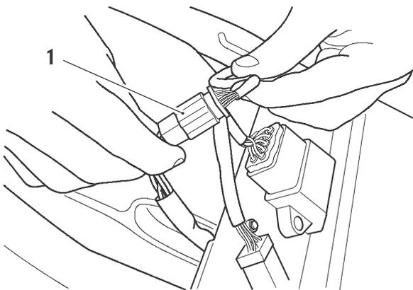
**1. Rear light unit wiring connector**
