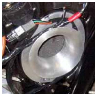
To take advantage of the improved airflow we increased the main jet size from 110 to 118 and put 2 shims under the needle. A visit to the Dynamometer at local racing team (Crescent Suzuki UK) resulting in the technician suggesting that another shim would be a good idea. So with 3 shims I thought it was going well. **Wrong!** The technician was used to working with fuel maps and doing everything with a computer: the bike still didn't run as I felt it should.
