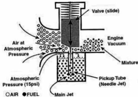
Both the CV and conventional slide carburetors, like Amals, are classified as variable venturi carbs. The slide on a conventional carburettor is directly connected to the throttle cable. Twist the throttle grip and the slide is raised in the venturi.
